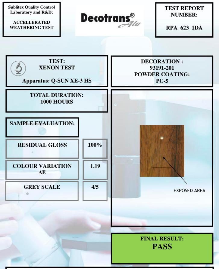
Test was carried on samples prepared according to technical specifications supplied by raw materials manufacturers. However, accelerated weathering test is only one of the conditions necessary for the evaluation of the finished product. For a final assessment see further analysis on natural exposure in Florida.
